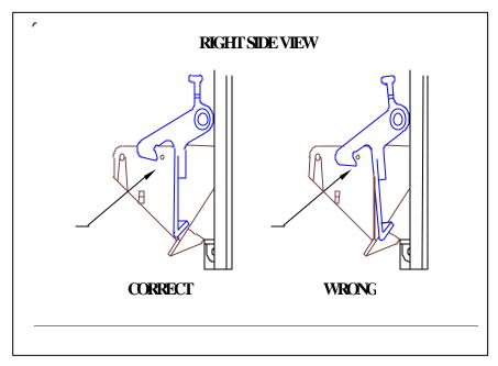
• Open and close the rack door to check the interface with the door tongue. Make sure that the right side of the tongue holds the coin retain door closed. Be sure that the tongue doesn't interfere with the coin deflector at the bottom of the mechanism.
