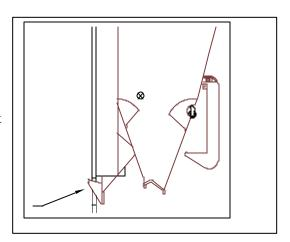
• The ST-110 rack section with the rack door closed. Note that the door tongue pushes the coin door closed.
