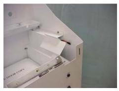
Installing the Lock Assembly
